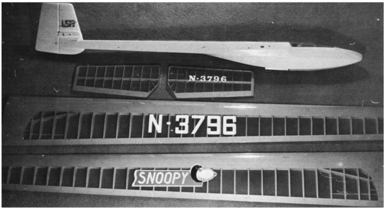
Snoopy's nose section. Note wing rod, band hold-down holes. Adjustable skid.
